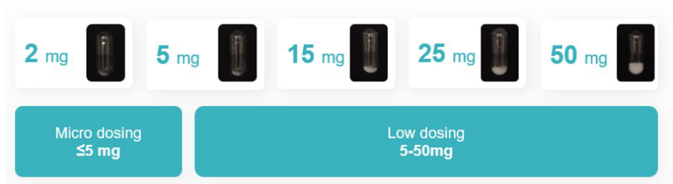
Figure 2: Standard capsules can be directly filled with pure active ingredient to create low-dose capsules, containing 5–100 mg. Microdose capsules contain less than 5 mg of active ingredient, which is often blended with just one nonfunctional filler material.
