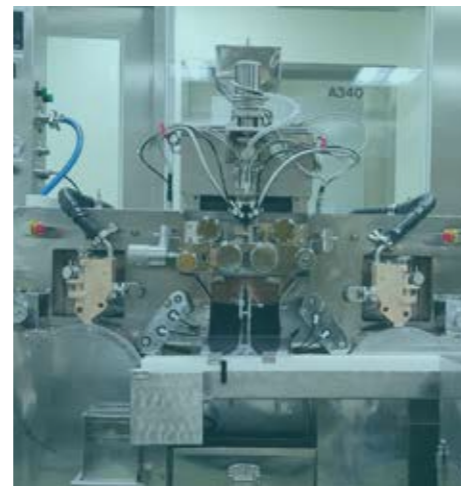
Figure 2 View of the central part of an SGC encapsulation machine
