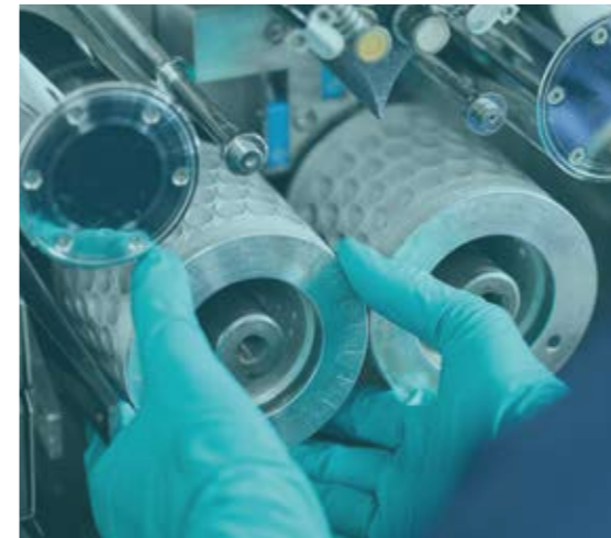
Figure 4 Assembly of the die rolls into the SGC encapsulation machine
